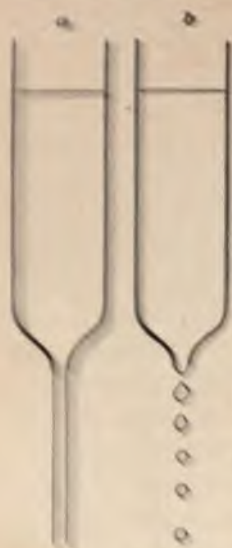
FIG. 12. Appearance of liquids of slight (a) and of great (b) surface tension when issuing from a glass tip.
